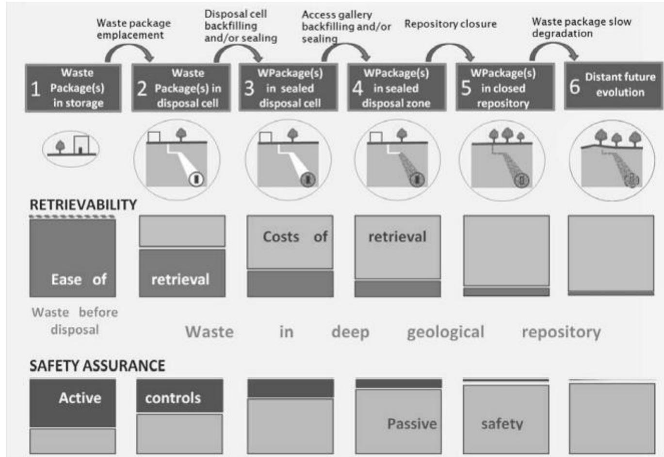
“R-scale” - Lifecycle stages of the waste, illustrating changing degree of retrievability, passive vs. active controls and costs of retrieval in a deep geological repository. During the operational phase, not all waste packages present in the facility will be at the same lifecycle stage.
