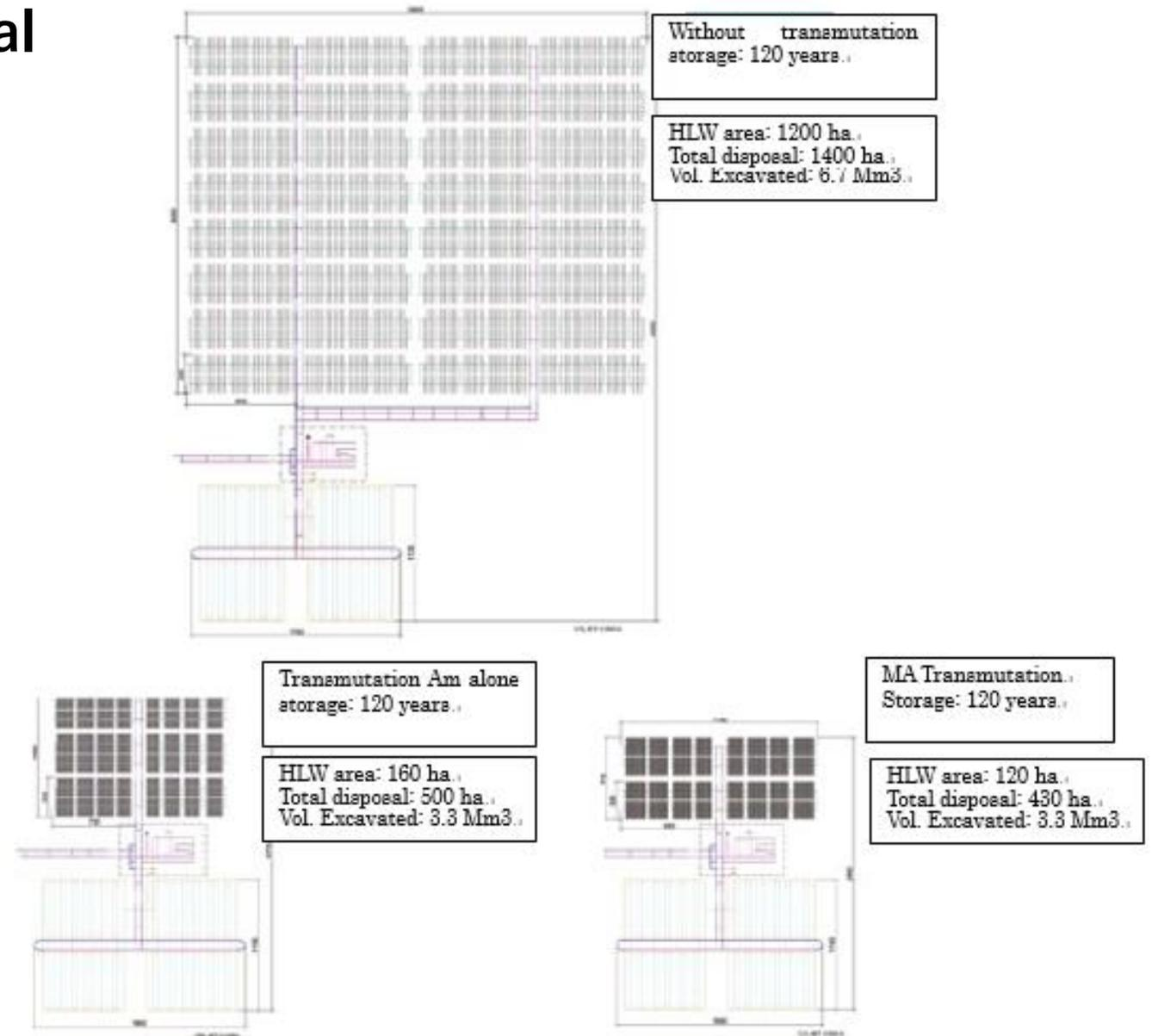
Figure 42: Comparison of underground disposal architectures for different scenarios of the 2012 study (single disposal for all the waste produced over the duration of the scenarios - 110 years of production)
