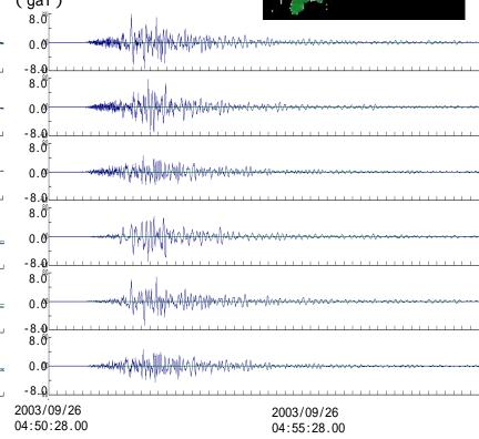
Sep.26, 2003, Main shock of "2003 off-shore Tokachi earthquake" M 8.0
