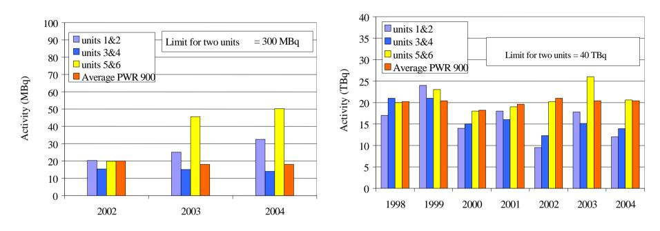
**Iodine release** Units 1-4 used MOX fuel Units 5-6 used only UOX fuel
