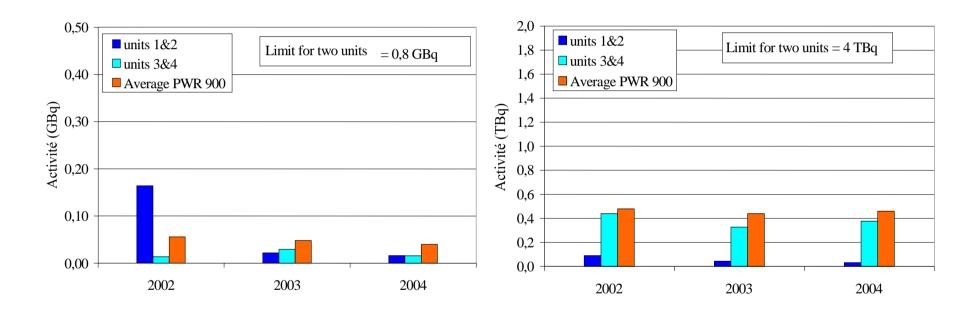
**Iodine release** Units 1-2 used MOX fuel Units 3-4 used only UOX fuel
