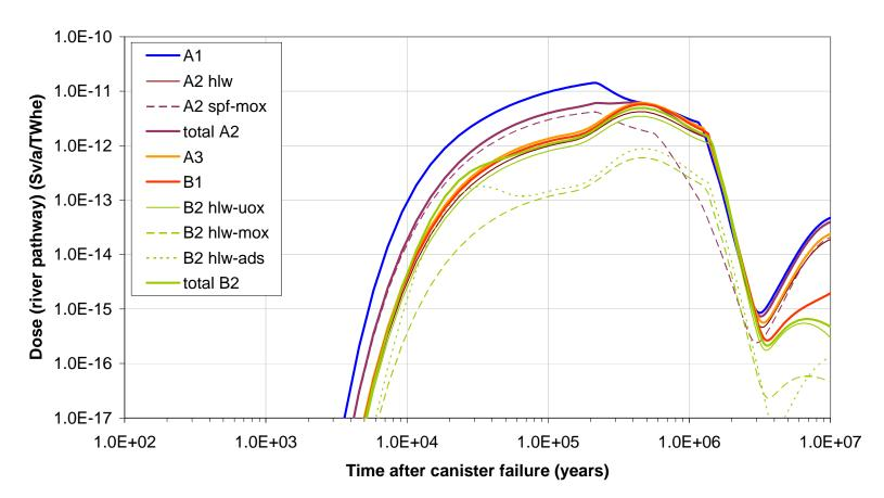
Impact of the various fuel cycles on the dose calculated for the normal evolution scenario:
