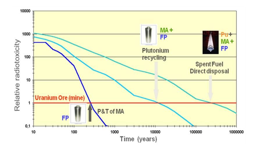
Simulation of radiotoxicity reduction vs. time (Ingestion radiotoxicity normalized to natural uranium and decay products as occurs in natural uranium ore).
