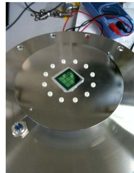
Field shaping rings are inserted between the cathode and the grid to maintain electric field.
