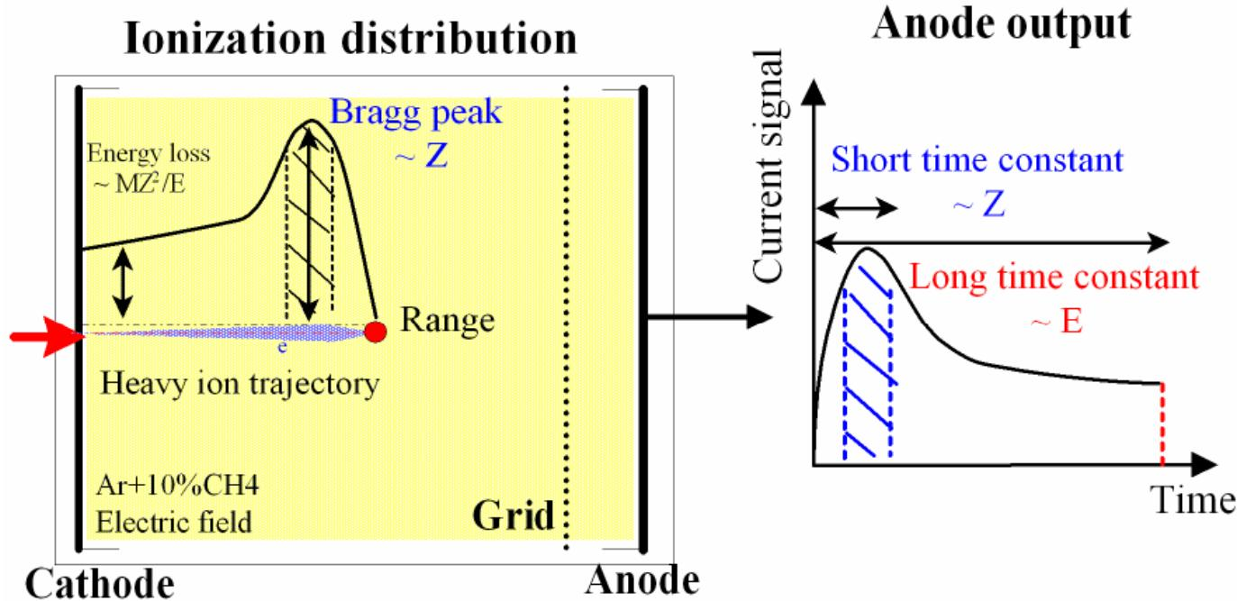
The electric field strength between the grid and the anode is more than four times of that between the cathode and the grid to lead all electrons to the anode electrode.
