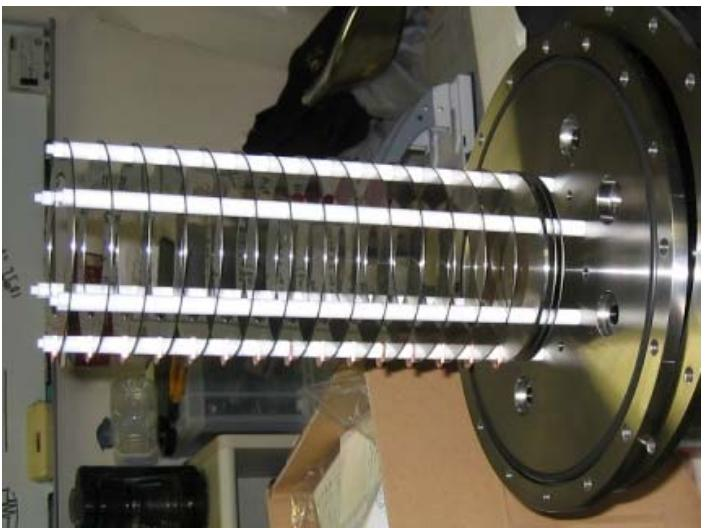
The BCC is a cylindrical chamber having a thin entrance window, cathode, grid and anode electrodes.
