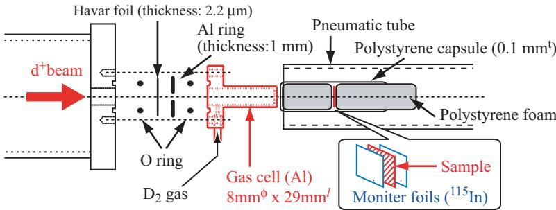
An expanded view around the gas target assembly. The target chamber consists of a small cell made of aluminum and filled with  $\text{D}_2$  at  $1.62 \times 10^5 \text{ Pa}$ . The samples were sandwiched between two indium foils of  $10 \times 10 \text{ mm}$  square and  $0.2 \text{ mm}$  thick, and were put in the sample cartridge. The indium foils of the  $^{115}\text{In}(n, n')$  reaction work as a neutron flux monitor.
