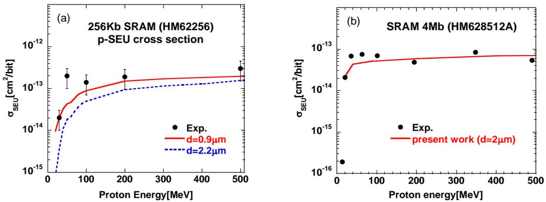
Fig.5 Comparison of calculated proton SEU cross-sections with experimental data [10,11]
