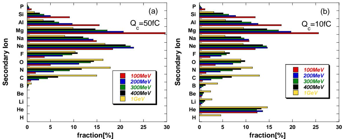
Fig.6 Relative contribution of each secondary ion to SEU cross section: (a)  $Q_c=50\text{fC}$  and (b)  $10\text{fC}$
