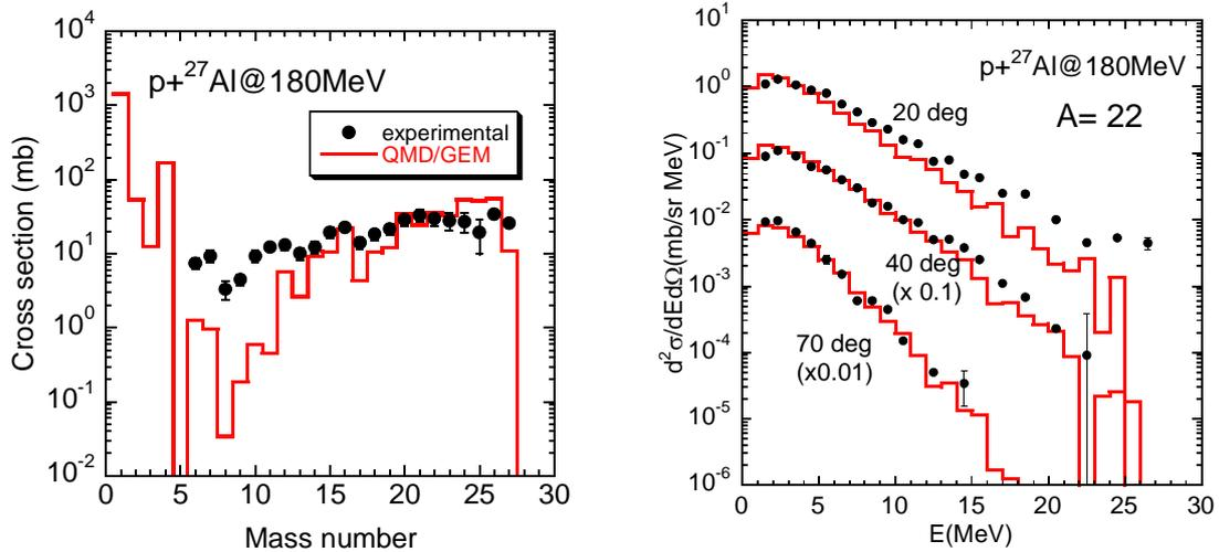
Fig.4 Comparison of JQMD/GEM calculation with experimental data of p+Al reaction at 180 MeV [7]
