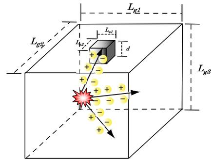
Fig. 3 Schematic illustration of memory cell geometry including the sensitive volume
