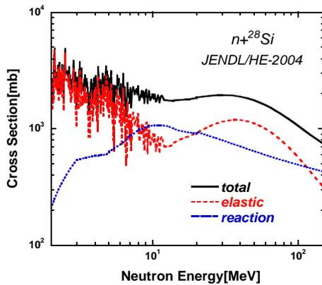
Fig.7 Neutron total, elastic, and reaction cross-section of  $^{28}\text{Si}$  taken from JENDL/HE-2004
