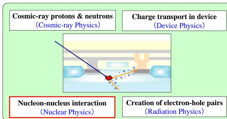
Fig.1 Schematic illustration of SEU phenomena
