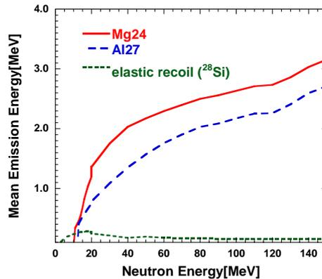
Fig.9 Averaged emission energy for elastic recoil ( $^{28}\text{Si}$ ),  $^{27}\text{Al}$  and  $^{24}\text{Mg}$
