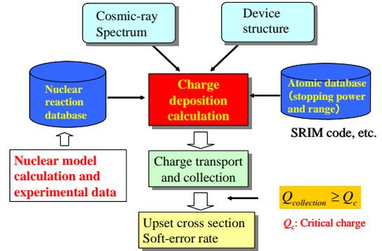
Fig. 2 Flow chart of SEU simulation
