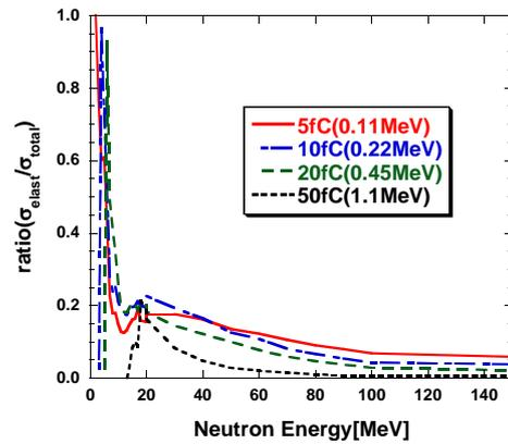
Fig.8 Ratio of the elastic SEU cross section to the total SEU cross section
