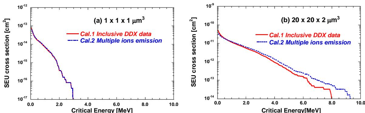
Fig.10 Calculated neutron SEU cross section as a function of critical energy  $E_c$  for the following sensitive volume: (a)  $V_s = 1 \times 1 \times 1 \mu\text{m}^3$  and (b)  $V_s = 20 \times 20 \times 2 \mu\text{m}^3$
