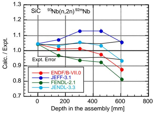
Fig. 1 C/E for reaction rate of  $^{93}\text{Nb}(n,2n)^{92m}\text{Nb}$  in SiC experiment.
