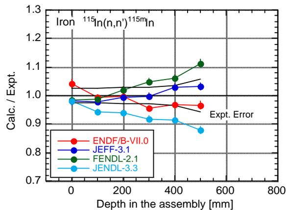
Fig. 6 C/E for reaction rate of  $^{115}\text{In}(n,n')^{115m}\text{In}$  in iron experiment.
