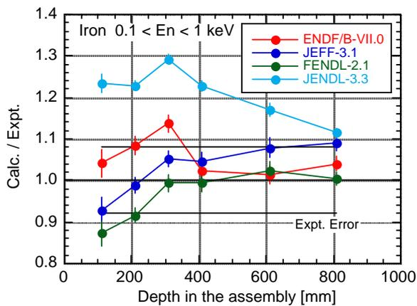
Fig. 5 C/E for neutron flux from 0.1 keV to 1 keV in iron experiment.
