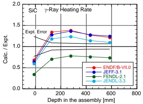
Fig. 2 C/E for gamma-heating rate in SiC experiment.
