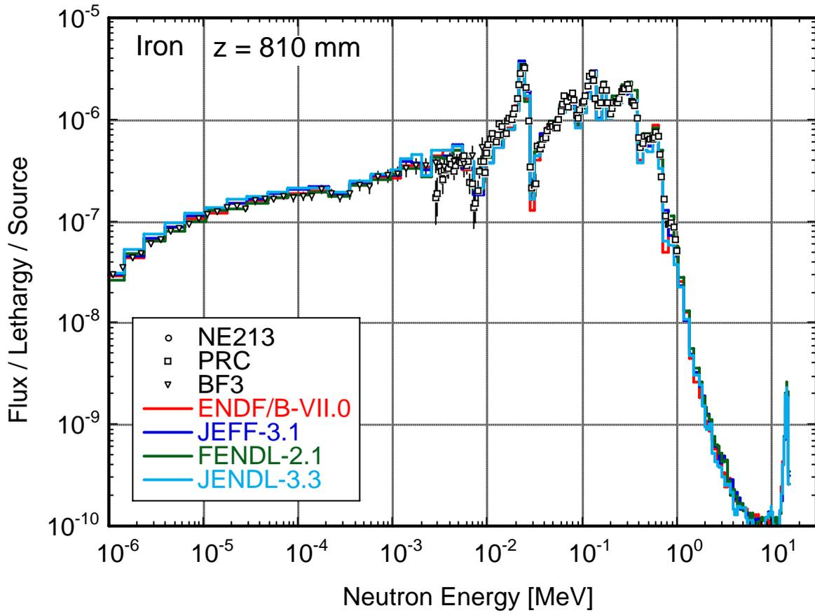
Fig. 4 Measured and calculated neutron spectra at depth of 810 mm in iron experiment.
