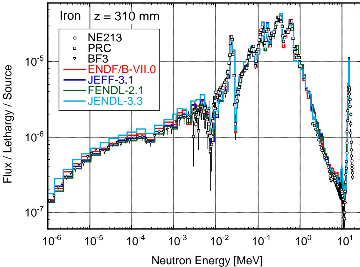
Fig. 3 Measured and calculated neutron spectra at depth of 310 mm in iron experiment.
