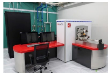
装置外観 (LEAP5000XR、CAMECA)
