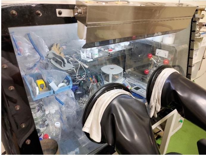
Fig1 : Use Glove Box to make SnBi alloy.
