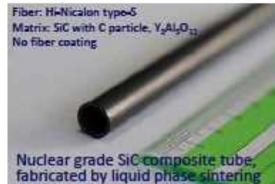
Nuclear grade SiC composite tube, fabricated by liquid phase sintering
