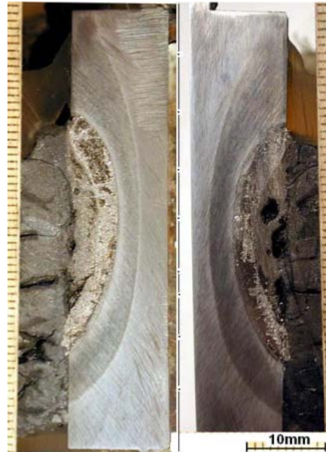
Axial section of a vertical specimen after interaction with an suboxidized melt
