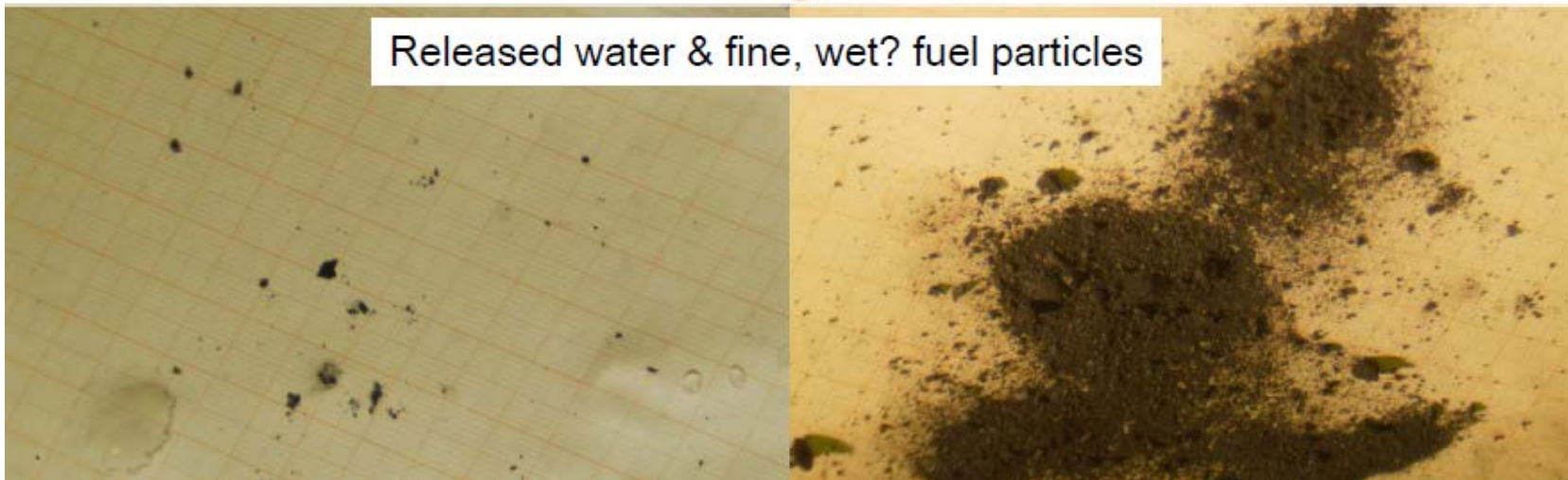
Figure; Fuel residue from posttest disassembly of IFA-650.9 (4)
