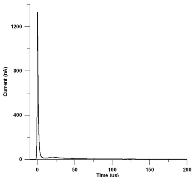
Figure 3. Response signal obtained at the San Raffaele hospital with the LINAC operating at 6 MV.
