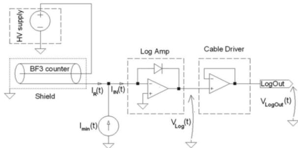
Figure 1. General scheme of the detector electronics.
