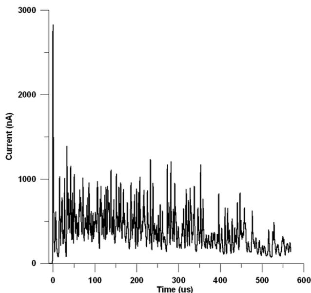
Figure 4. Response signal obtained at the San Raffaele hospital with the LINAC operating at 18 MV.
