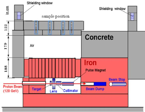
Figure 1. Cross sectional view of the Pbar target station.
