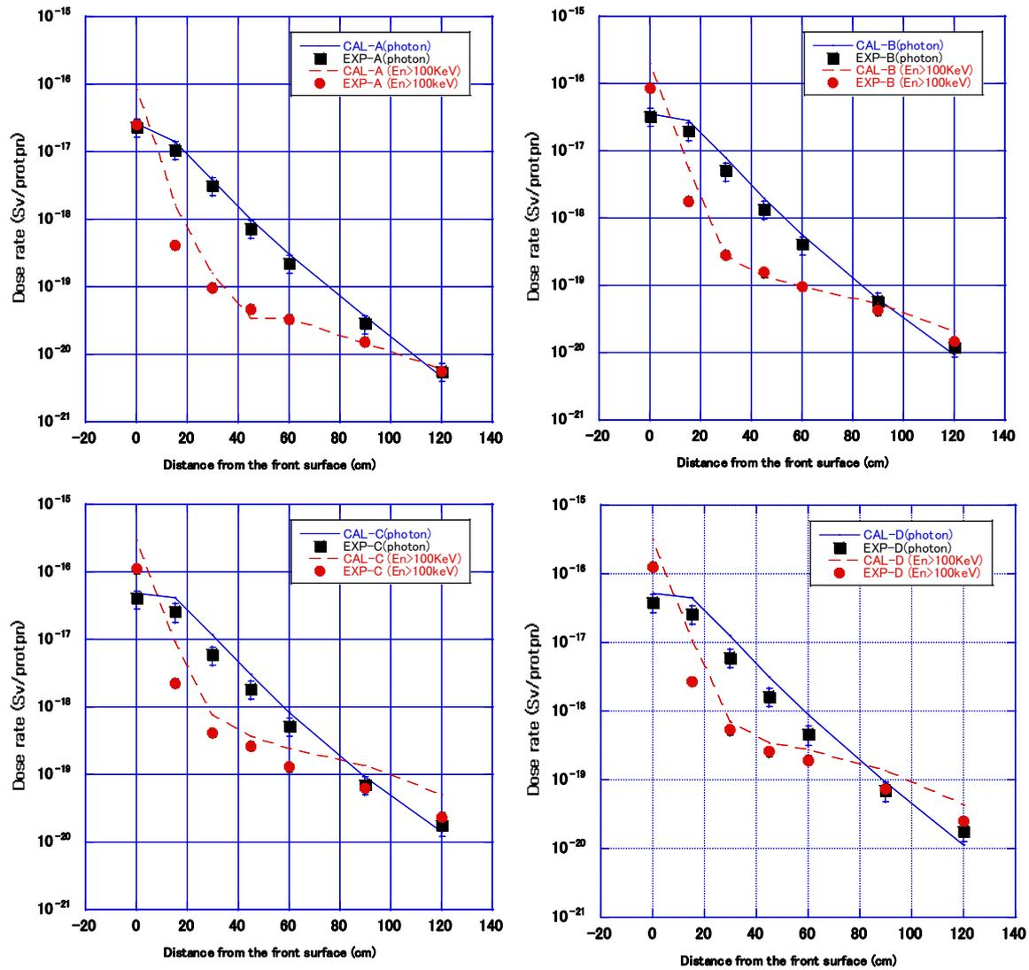
Figure 4. Experimental and calculated results of dose rate for each experimental hole.
