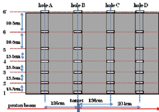
Figure 2. Positions of installed detectors in concrete shields.
