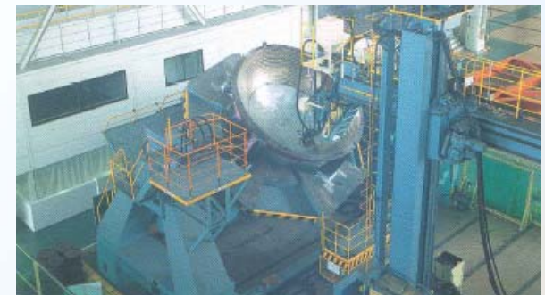
Dome Cladding Equipment
