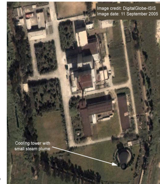
New satellite image of the 5 MWe reactor at Yongbyon, North Korea that shows a steam plume from the cooling tower. This plume indicates that the reactor is operating.
