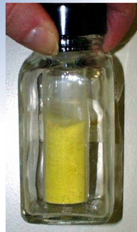
High purity uranium oxide product recovered from used nuclear fuel using the UREX+ process
