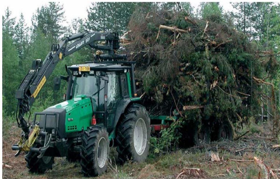
Figure 37. Valtra farm tractor-based residue forwarder of Metsäenergia with enlarging load space (TTS Institute).
