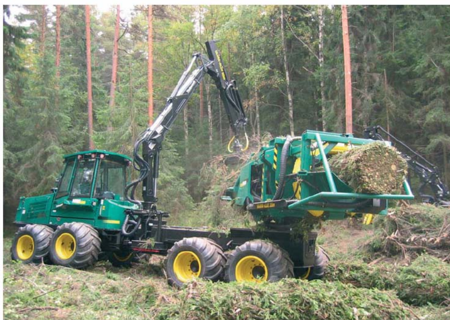
Figure 30. Timberjack 1490D baling logging residues of spruce (Timberjack).
