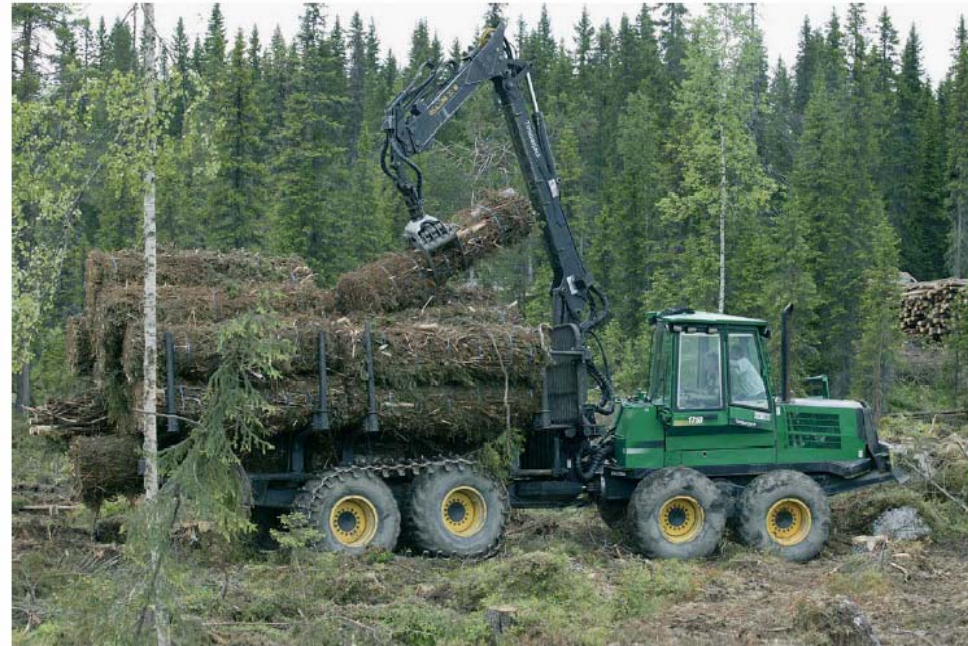
Figure 31. Conventional Timberjack 1710 forwarder unloading compacted residue logs at road side (Timberjack).
