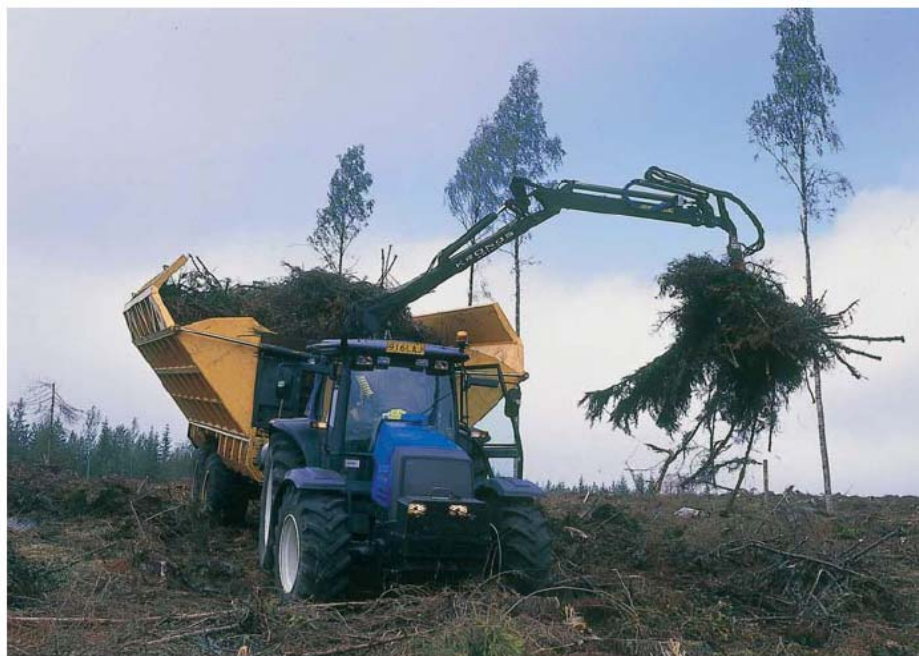
Figure 34. Load-compacting HavuHukka forwarder for transporting logging residues from stump to satellite terminals (Vapo).
